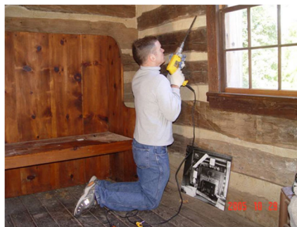
Henderson taking wood samples to determine a building's date.
